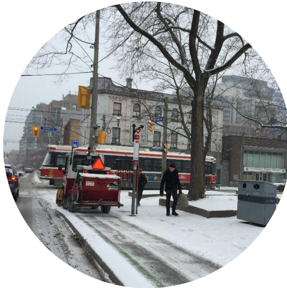
SIDEWALK PLOW CLEARING A VERTICALLY SEPARATED CYCLE TRACK Location: City of Toronto
