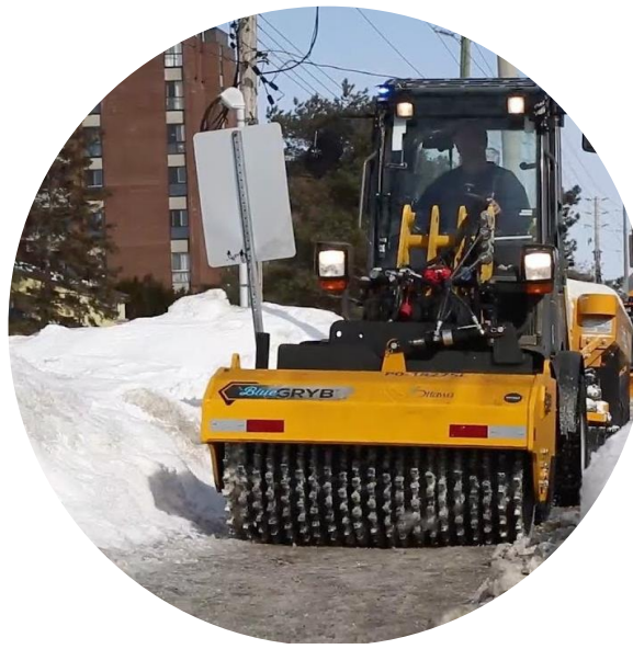
BLUE GRYB ROTATING ICEBREAKER CRUSHING ICE ON A SIDEWALK Location: City of Montreal
