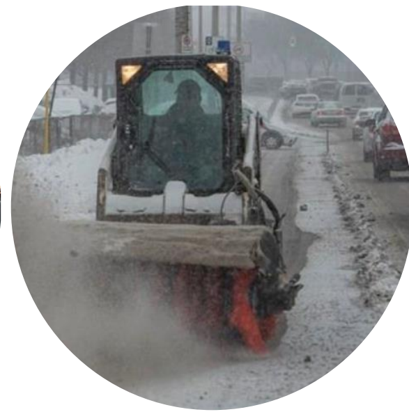
WINTER MAINTENANCE VEHICLE WITH BRUSH ATTACHMENT Location: City of Hamilton
