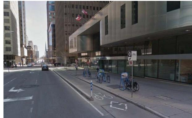
Figure 72: Example of existing separated bike lanes with pre-cast concrete curbs on Laurier Avenue, Ottawa
