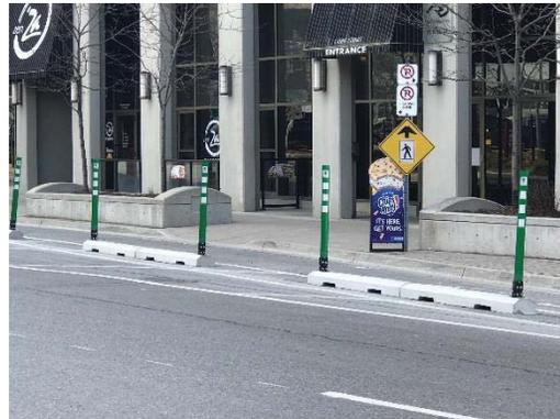
Figure 71: Example of existing separated bike lanes with flex bollards in London, ON
