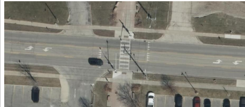
Figure 16: Mid-block crossing along County Road 20 and off-road multi-use trail, Leamington Source: Google StreetView
