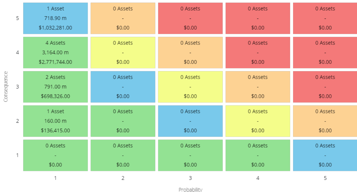
Figure 6-3: Stormwater Network Risk Matrix
